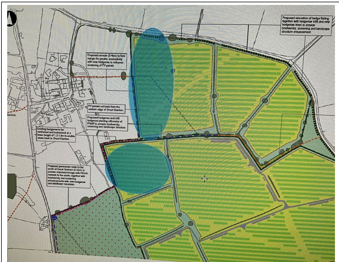
Panel Area D , blue lozenge shapes are priority areas that RWE has proposed for removal subject to improved technology such as more efficient panels being available at the point of detail design.
